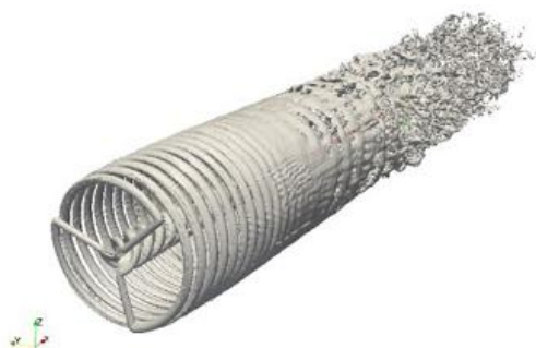
Fig. 17 Vortex isosurface contours and wakes structure
