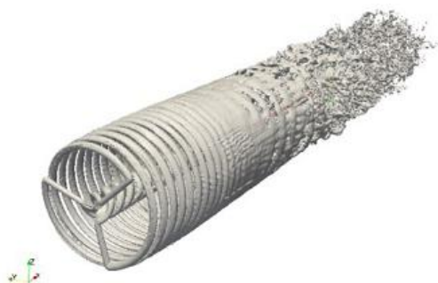
Fig. 17 Vortex isosurface contours and wakes structure
