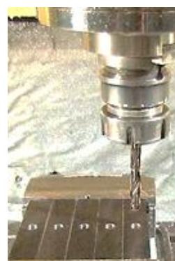
Fig. 2 Drilling of fatigue test specimens
