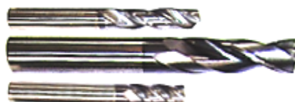
Fig. 1 Carbide drills and end mill used in tests
