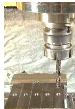
Fig. 2 Drilling of fatigue test specimens
