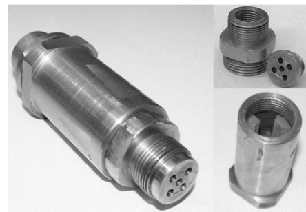
Fig. 6 Components of test motor's igniter
