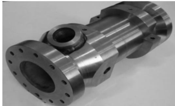
Fig. 8 Gas generator's mass-launcher with igniter location
