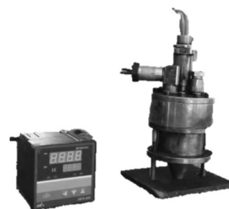
Fig. 10 Propellant's test motor with temperature indicator, sensors and other accessories
