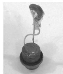
Fig. 7 Initiator of test motor's igniter
