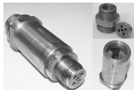
Fig. 6 Components of test motor's igniter
