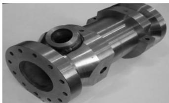
Fig. 8 Gas generator's mass-launcher with igniter location
