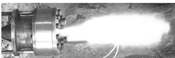
Fig. 16 Test of propellant with HTPB binder
