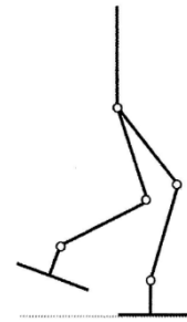
Fig. 2 Robot model in single support phase (open kinematic chain)
