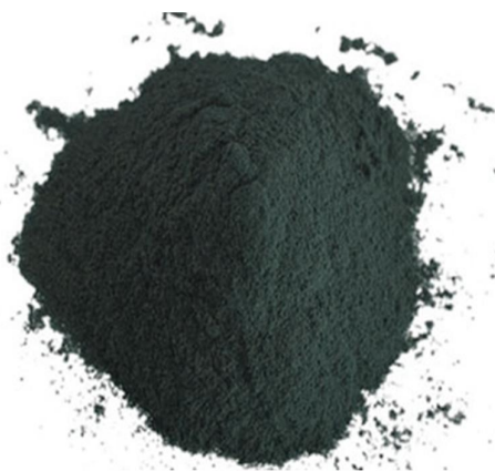
Fig. 4 the PP/AGO nanocomposite powder
