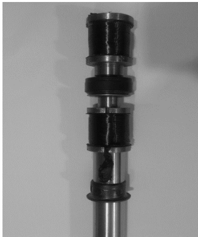
Fig. 9 Set of control valve
