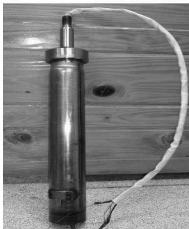
Fig. 10 The final MR damper fabricated
