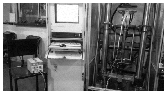
Fig. 11 A view of fabricated MR damper under damping test
