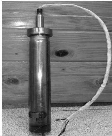
Fig. 10 The final MR damper fabricated
