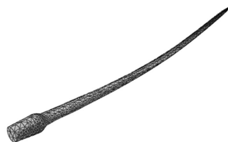
Fig. 11 The first bending mode of turbine blade vibration in ABAQUS software
