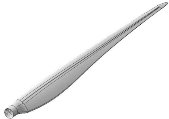
Fig. 3 The blade of 5-MW wind turbine with various property in length in CATIA software
