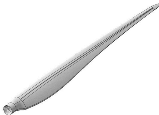
Fig. 3 The blade of 5-MW wind turbine with various property in length in CATIA software
