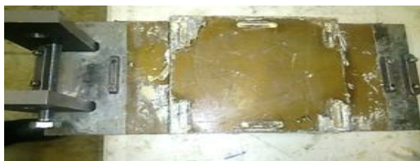
Fig. 2 Mould Manufacturing of fiber metal laminate
