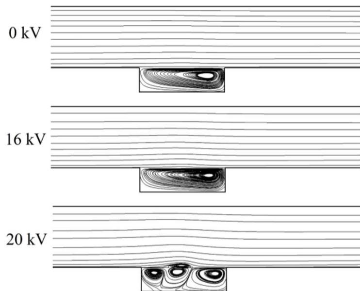
**Fig. 11** Streamline for different applied voltages: Re=18652
