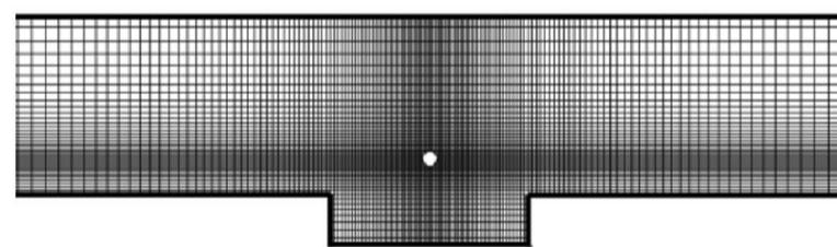
**Fig. 3** 2D view of computational grid
