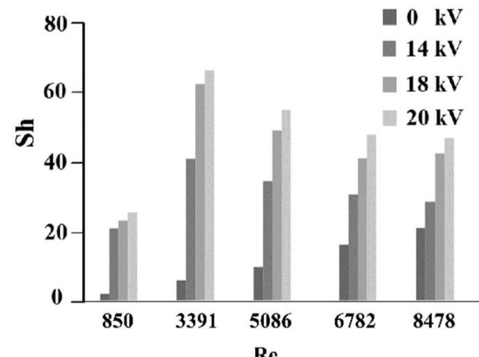
**Fig. 12** Sherwood number versus Reynolds number and applied voltage
