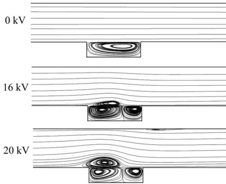
**Fig. 10** Streamline for different applied voltages: Re=8478
