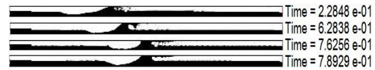
Fig. 3 Mesh independency of slug regime in channel flow with k-ε RNG turbulent model
