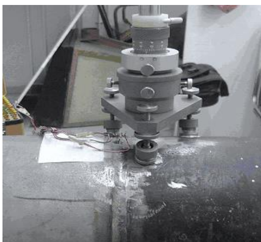
Fig. 2 Residual stress measurement by the hole drilling technique
