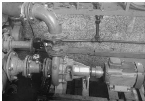
Fig. 3 Test Setup of Centrifugal Pump
