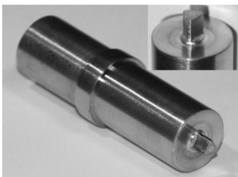
Fig. 2 The FSW tool used for all the welding processes
