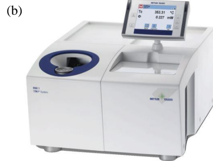
Fig. 4 a- DSC test results and adopting phase transformation temperatures from the Heat Flow-Temperature diagram, b- DSC test setup
