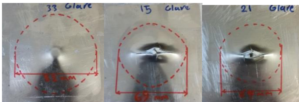
Fig. 19 Damage zone propagation on target No.33 (flat projectile), No.15 (hemispherical projectile) and No.21 (conical 90° projectile)
