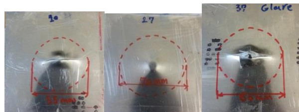
Fig. 13 Damage zone propagation on target No.10 (hemispherical projectile), No.27 (flat projectile) and No.37 (conical 90° projectile)
