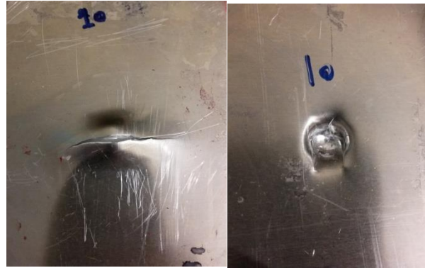
Fig. 11 Target No.10: front side (left) and back side (right) view under the penetration of hemispherical projectile in 40J impact
