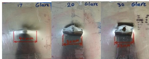
Fig. 26 Bottom layer of aluminum 2024 tear on specimen No.17 (flat projectile), No.20 (hemispherical projectile) and No.30 (conical projectile) in 70J impact.
