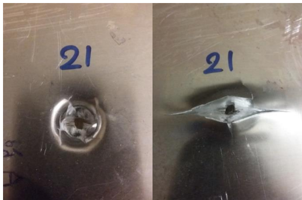
Fig. 18 Target No.21: front side (right) and back side (left) view under the penetration of conical 90° projectile in 55J impact
