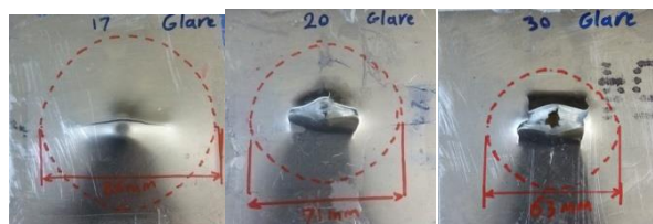
Fig. 25 Damage zone propagation on target No.17 (flat projectile), No.20 (hemispherical projectile) and No.30 (conical projectile)
