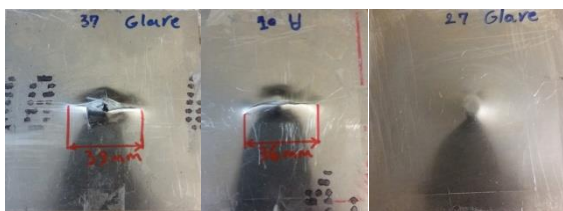
Fig. 14 Bottom layer of aluminum tear on specimen No. 27 (flat projectile), No. 10 (hemispherical projectile) and No. 37 (conical 90° projectile) in 40J impact.
