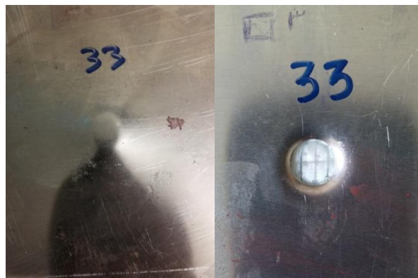
Fig. 16 Target No.33 front side (left) and back side (right) view under the penetration of flat projectile in 55J impact
