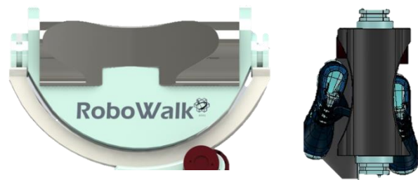
Fig. 4 Ergonomic design of RoboWalk's seat Right) Top view orientation Left) Right view orientation
