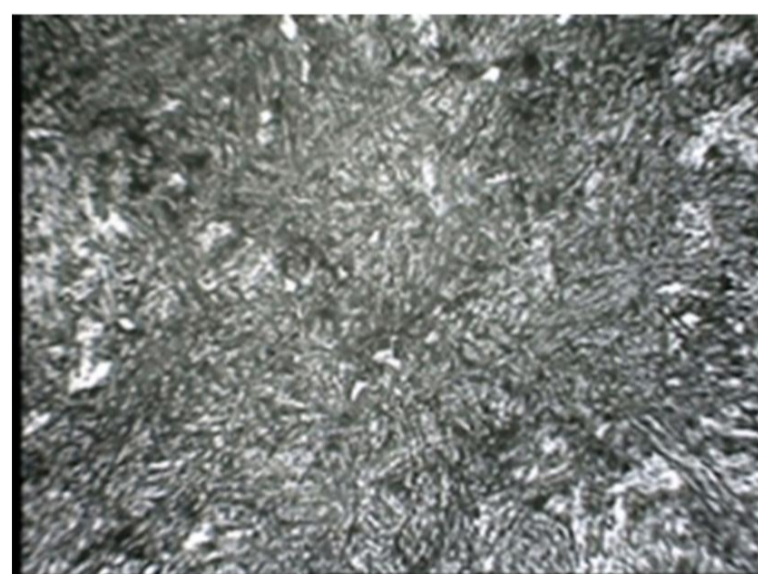
Fig. 5 The micro structure of the bainite phase
