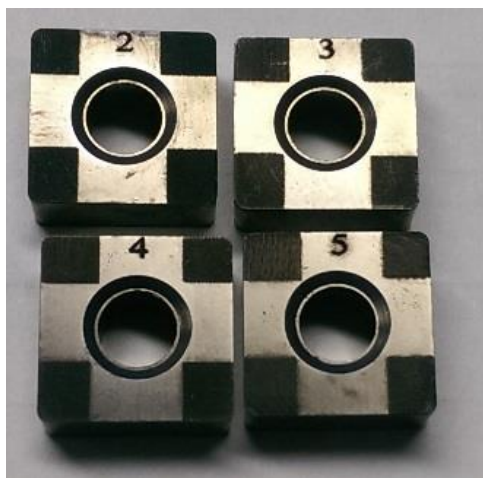
Fig. 4 Cutting inserts after creating the micro-texture
