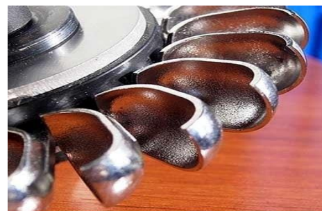
Fig. 2 The blades of Turgo turbine [33]
