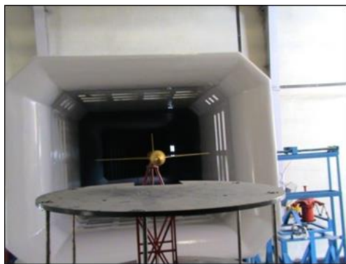
Fig. 17 Delta wing airplane model installation on ground simulation stand ( H/b=0.2 )
