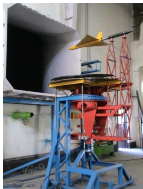
Fig. 15 Delta wing airplane model installation on ground simulation stand
