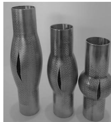
Fig. 19 Experimental bulged components for the effect of different lengths in free bulge (r=5 mm)
