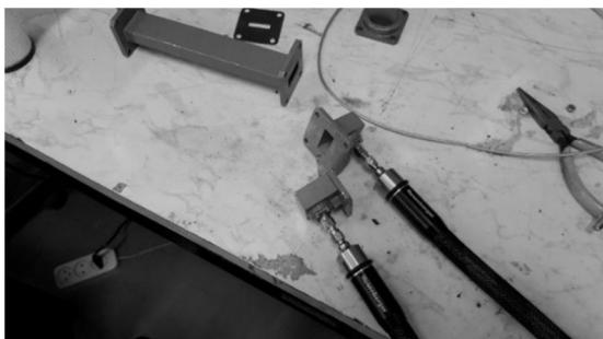
Fig. 9 A view of Short Load calibration step
