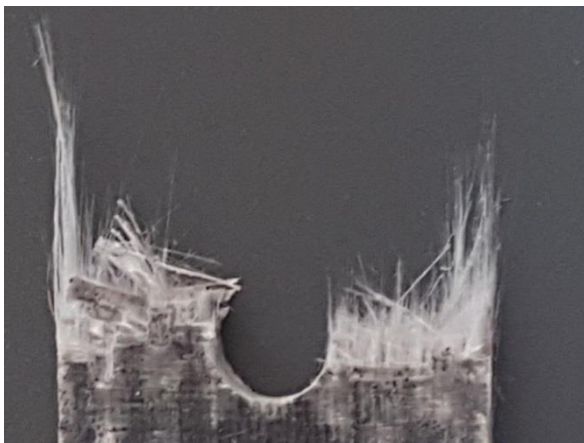
Fig. 9 Failure area in specimen with 0.5 percent carbon nanotube after fatigue loading
