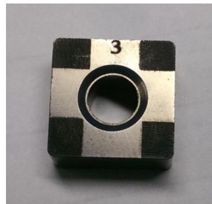
Fig. 4 Cutting insert image after creating the micro-texture
