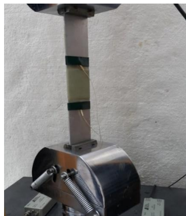
Fig. 2 Tensile test of reinforced specimen with composite patch
