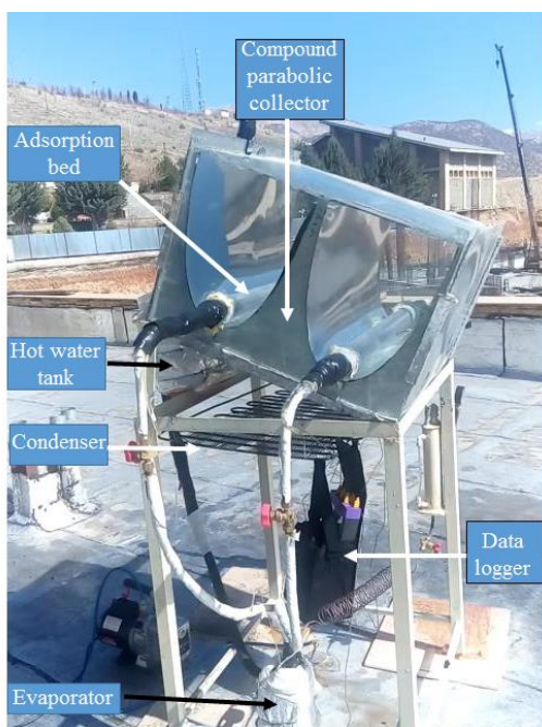
Fig. 1 two bed solar adsorption chiller
