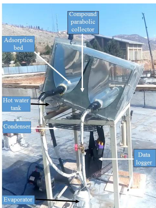
Fig. 1 two bed solar adsorption chiller
