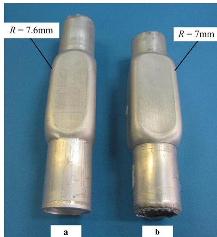
Fig. 11 Work pieces obtained at different pressure applying time (a) Time 30s (b) Time 90s
