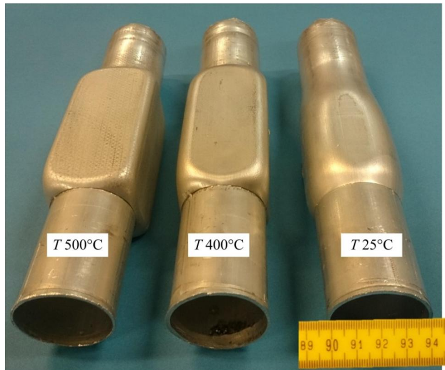
Fig. 5 Square specimens shaped in different temperature
