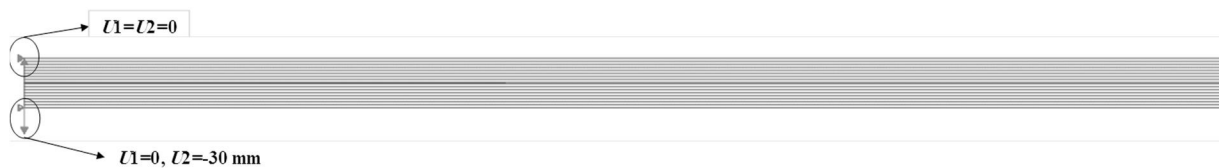
Fig. 6 DCB specimens boundary conditions
