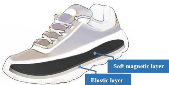
Fig. 11 A smart sensing insole engaging all-around magnetic layer
