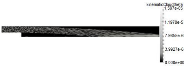
Fig. 11 The volume ratio of particles to the fluid around (gas) after one second in the step problem
