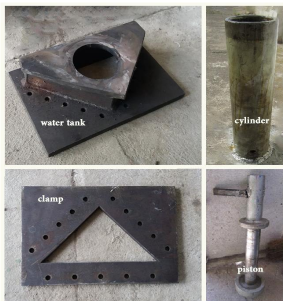
Fig. 1 schematic view of deformation system
