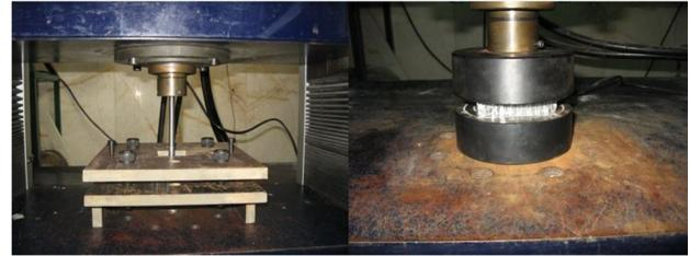
Fig. 4 Universal testing machine used in concentrated and distributed loading quasi-static tests
