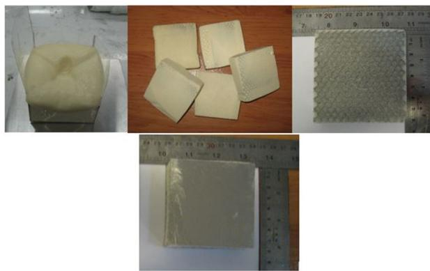
Fig .3 Preparation of sandwich panels filled with foam
