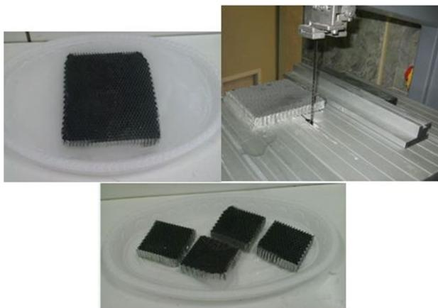
Fig.2 Preparation and cutting of honeycomb structures
