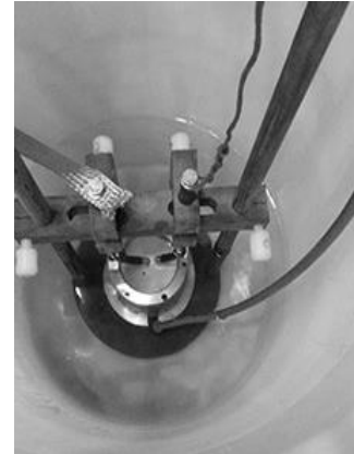
Fig. 5 Electrode system in the water chamber
