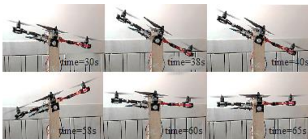
Fig. 17 Neuro controller response on real system
