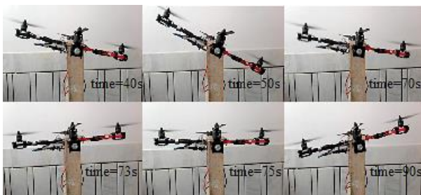
Fig. 16 PD controller response on real system
