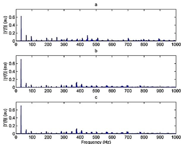
**Fig. 11** Fourier spectra for: a) Normal condition. b) Misalignment fault condition. c) Unbalance faulty condition
