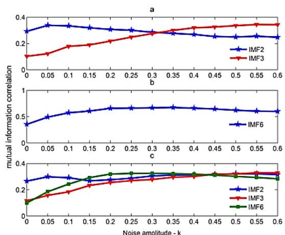
**Fig.4** The mutual information coefficient of the most important IMFs with the original signal for different amplitudes of the added noise. a) Normal condition. b) Misalignment fault condition. c) Unbalanced faulty condition.(In order to avoid the figure bustling, only IMFs with maximum mutual information coefficients are plotted)
