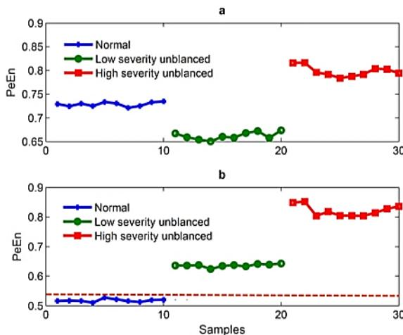
**Fig. 10** The PeEn values a)For the original signals. b) For the second IMF; the first 10 samples are in normal working conditions, the second 10 samples are in low severity unbalanced and the rest 10 samples are in high severity unbalanced working conditions.
