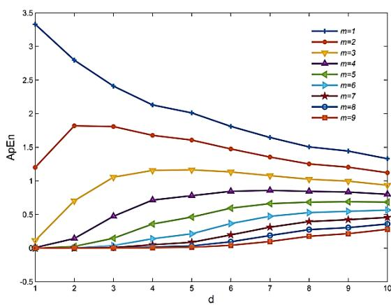
Fig. 3 ApEn values of normal vibration signal versus m and d variation
