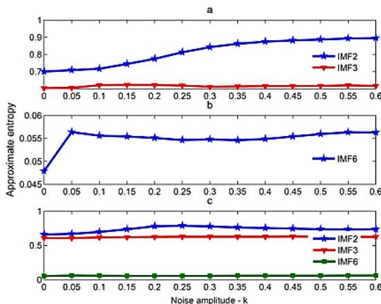
**Fig. 5** The ApEn values of the most important IMFs with the original signal for different amplitudes of the added noise. a) Normal condition. b) Misalignment fault condition. c) Unbalanced faulty condition
