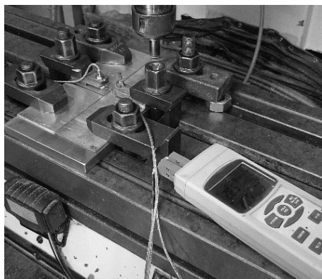
Fig. 3 Temperature measuring mechanism
