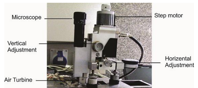
Fig. 2 The device used for high-precision stage punching
