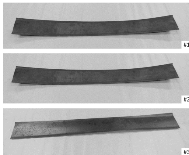
Fig. 8 Schematic of deformed sheet of Alform 700 M
