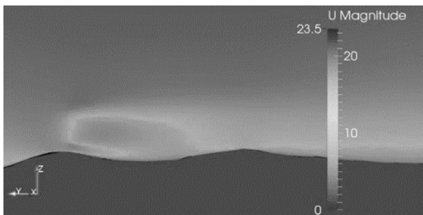
Fig. 6 Wind speed (m/s) of T5 wake in the Manjil wind farm
