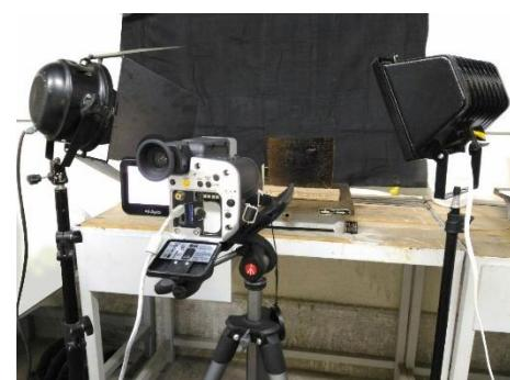
Fig. 4 Experimental set-up used to thermography
