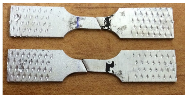
Fig. 2 fracture of sample after uniaxial tensile test
