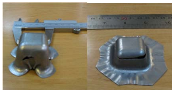
Fig. 15 Comparison of Al(0.4mm)/St(1.6mm) sheet forming with traditional (left) and hydromechanical (right) methods
