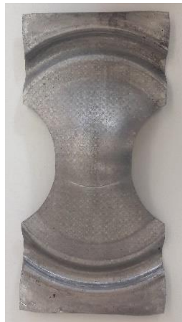
Fig. 5 sheet sample after necking
