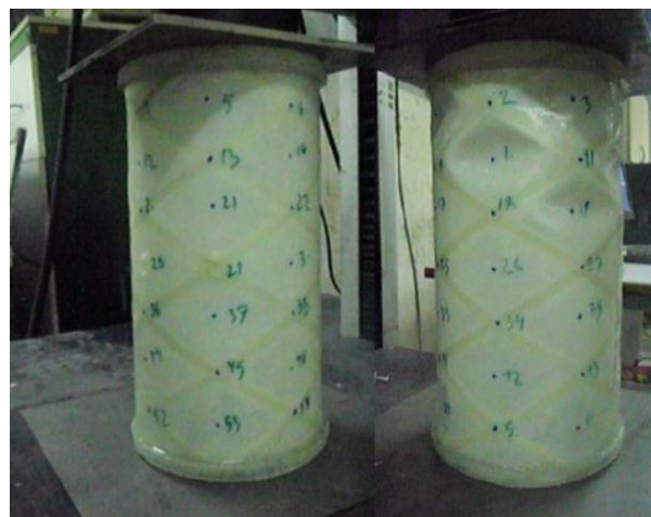
Fig. 12 Specimen before and after buckling
