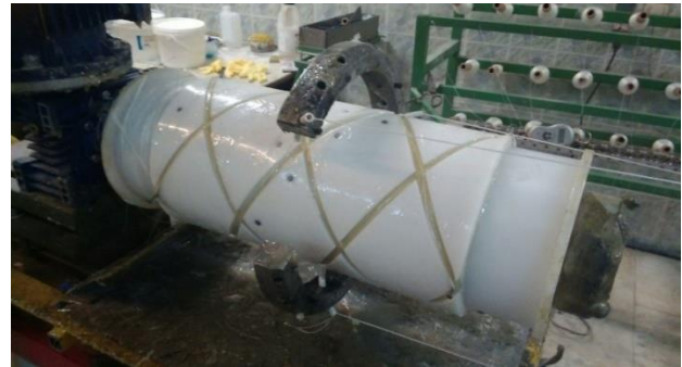
Fig. 5 Fabrication process of stiffeners
