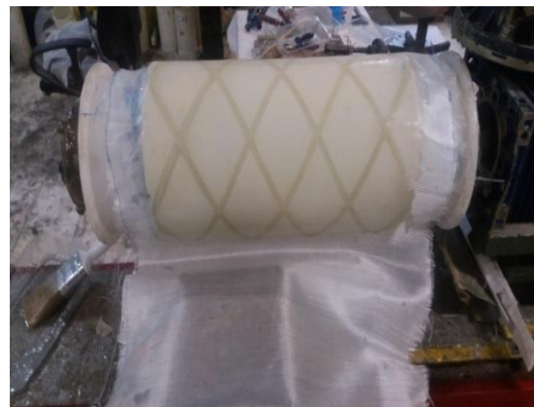
Fig. 6 Fabrication process of specimens
