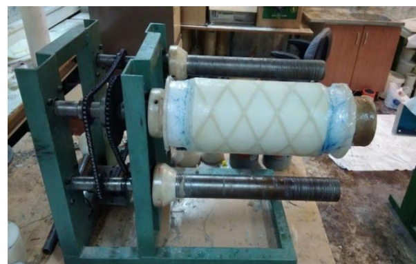
Fig. 7 Resin curing &amp; distribution process
